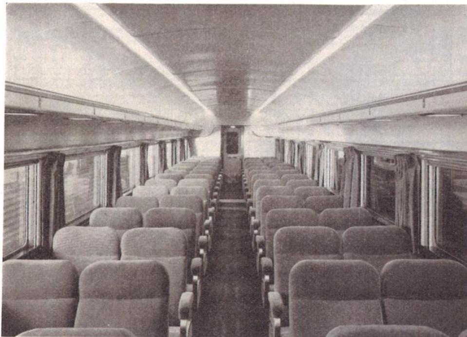
One of the Coaches — Indirect Light from the Ceiling is Supplemented by Prismatic Lights under the Luggage Racks
